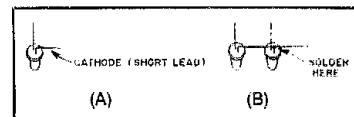
Fig. 10 — (A) The minutes and seconds LED cathodes are bent in this shape prior to mounting. (B) Each cathode of a 10-LED group is soldered as illustrated.
