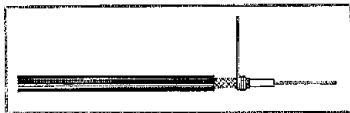
Fig. 2 — You can make a neat connection to the shield braid on a piece of Teflon-dielectric miniature coaxial cable by wrapping a few turns of wire around the braid and soldering it.
