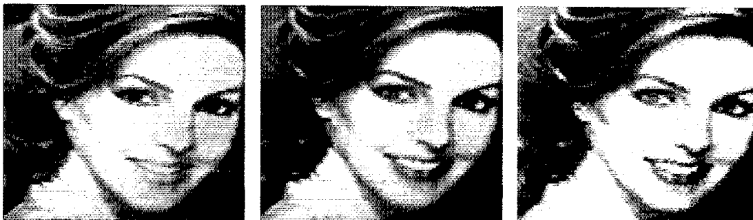
Fig. 1 — An RGB frame-sequential color SSTV picture received from KC5VC on 14.230 MHz. From left to right are the red frame in B & W, the red and green frames combined and the full-color RGB composite picture. (photos by George Switt, W8AMB)
